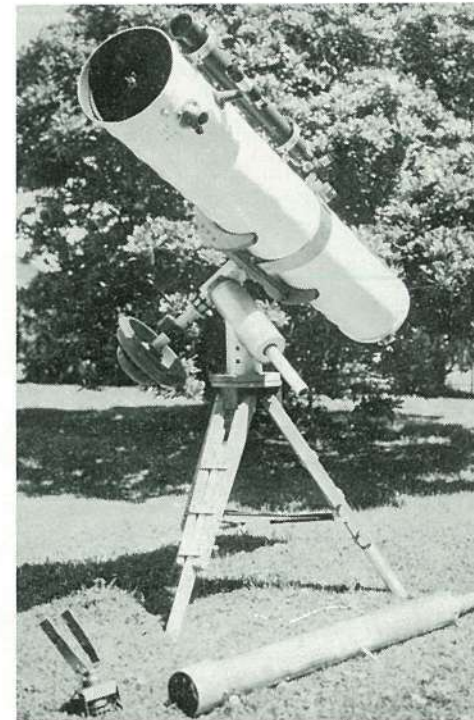
Chris Fuller's Home-built Reflecting Telescope
